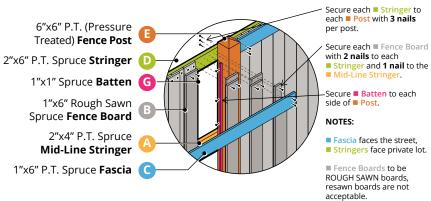
Noise Attenuation Fence is similar to a typical wood screen fence EXCEPT for a doubled up, staggered row of ■ Fence Boards; a wider ■ Bottom Stringer that is flush to the final grade; and ■ Battens secured to each post. There are to be NO gaps in this fence.
